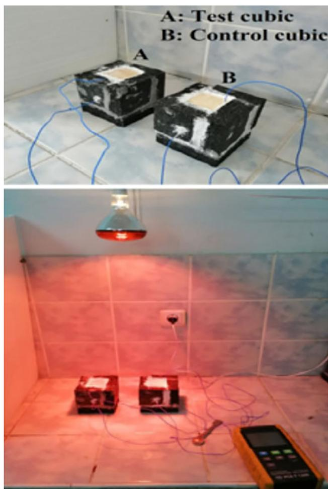
**FIGURE 1** Lab-scale cubic designs constructed for the estimation of thermo-regulative performance of the PCM impregnated wood [Colour figure can be viewed at [wileyonlinelibrary.com](http://wileyonlinelibrary.com)]
